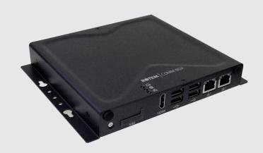
The Munters Rotem Comm-Box supplies complete web access with remote monitoring and control for your Rotem livestock controller from any internet-connected device with a web browser.
