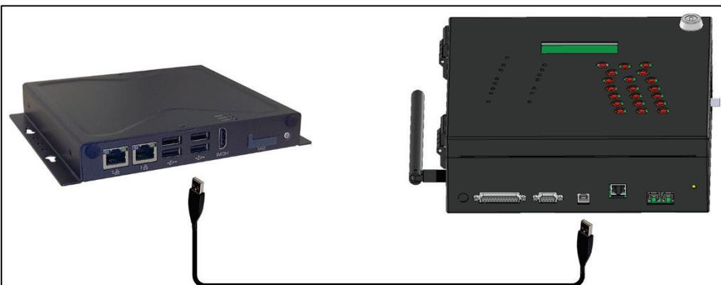
*NOTE Communicator requires the Communicator Serial Card (P/N: C-COMM-SERIAL) to support the Comm-Box. Refer to Document #112189 for details on upgrading the Communicator.*
