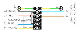
Anti—clockwise rotation (looking in the airflow direction)
