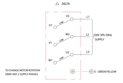
Replace the terminal cover and test run the fan unit, checking the rotation and fan currents.
