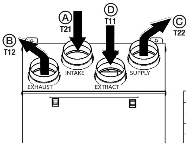
Fig. 7.a QR280E temperature probes.
