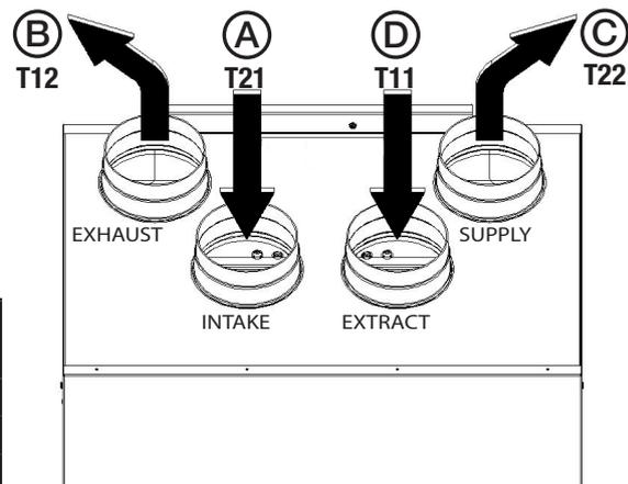
Fig. 7.b QR590E temperature probes.
