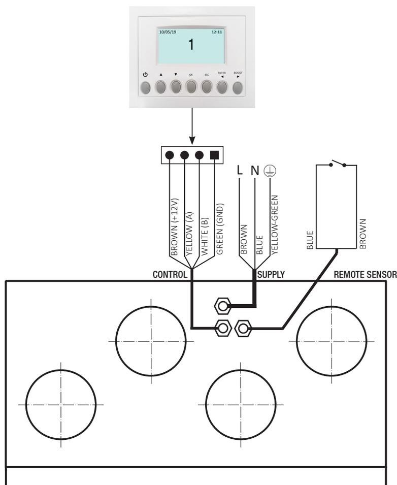
**Fig. 5.p** Electric connections
