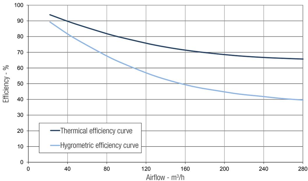
**Fig. 6.b** Data of the enthalpic heat exchanger.
