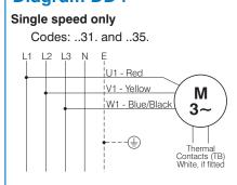
\*Additional Information: Refer to the motor manufacturer's data on the motor for wiring diagrams on standard frame Ex e, Ex d etc. motors.
