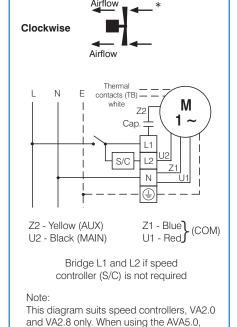
VA5.0 and VA8.0 speed controllers, use the AUX, MAIN and COM connections.
