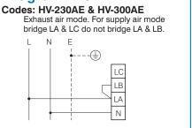
These diagrams are current at the time of publication, check the wiring diagram supplied with the motor.
