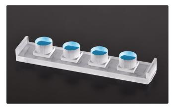
HoloLid placed in a Sarstedt lumox® multiwell 24 plate (right). The areas marked blue are the observation windows which are immersed into the cell media (right).
