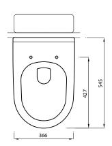
**Special notes**Pan fixes to floor using side fixing bracket supplied with pan.
