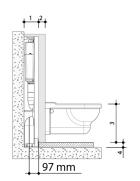
$1 = 142/147 \sim 245 \text{ mm}$   $2 = 16 \sim 100 \text{ mm}$  $4 = 0 \sim 200 \text{ mm}$
