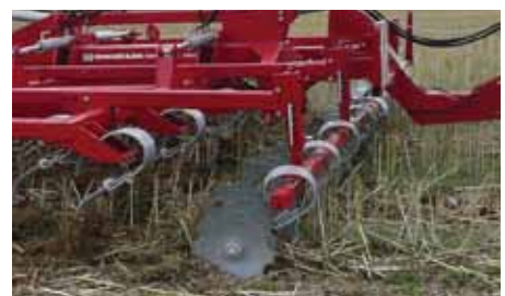
Front disc section - Vibro Flex 7400.
