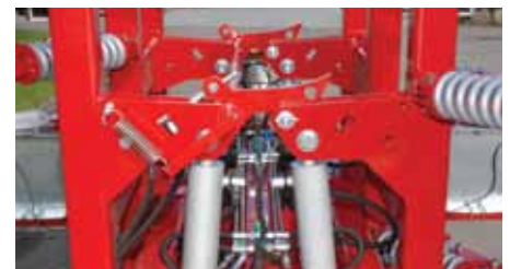
Automatic hydraulic wing lock system.
