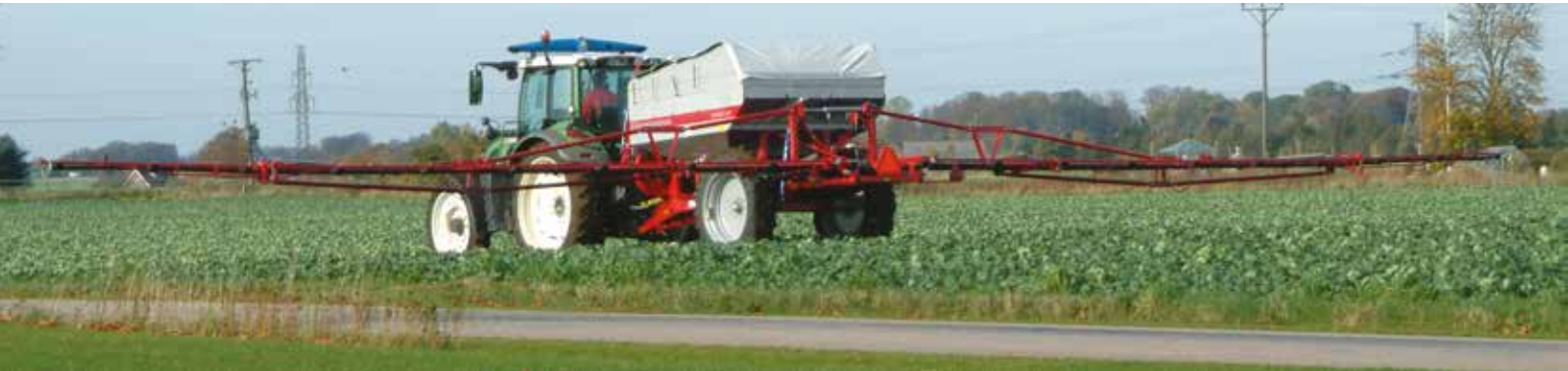
Kongskilde Wing Jet S 4824 K-Plus Hydro working in tramlines. Full application rate all the way to the edge.
