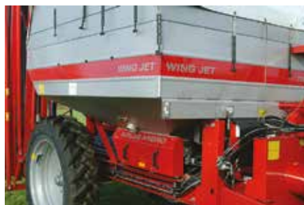
The hydraulic motor, powered by the tractor hydraulic system, is precisely controlled from the K-Plus and the proportional valve. The ground speed is recorded from a wheel sensor.
