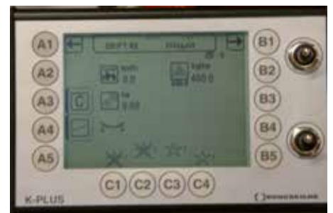
From the K-Plus monitor the operator can control the Wing Jet and receive information and alarms. With connection cables the control of sections on/off, and application rate settings can be taken over by GPS or N-Sensor.
