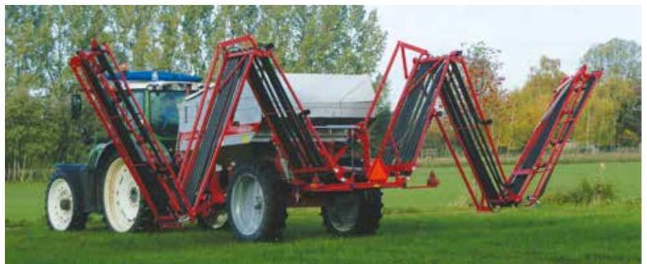
Easy hydraulic boom folding.
