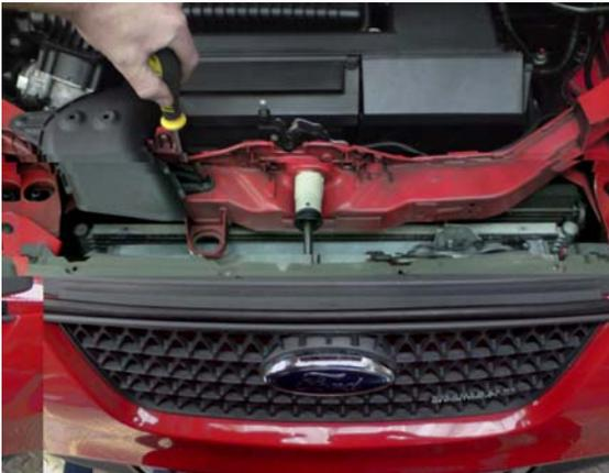
3. Remove ECU cover, this will slide upwards and then out.
