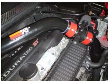
**TIP:** *Before fitting the air filter, there is a small plastic shield that is situated in the near side of the bumper next to the intercooler, we suggest that you take this out as it improves air flow to the filter.*
