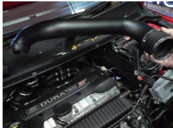
**15.** Check that all the bolts and brackets are present in the kit; fit the new DS Ind kit pipe into the turbo tube.
