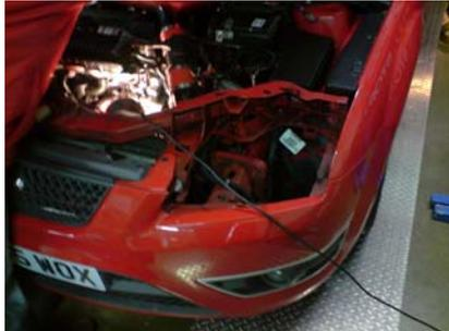
**23.** Insert the second pipe down past the ECU and the nearside chassis leg and secure to the chassis using the supplied bracket, this will mount on and existing captive nut attached to the chassis leg. (Do not tighten, at this stage).
