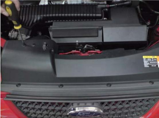
2. Extract three screws for air intake and remove.
