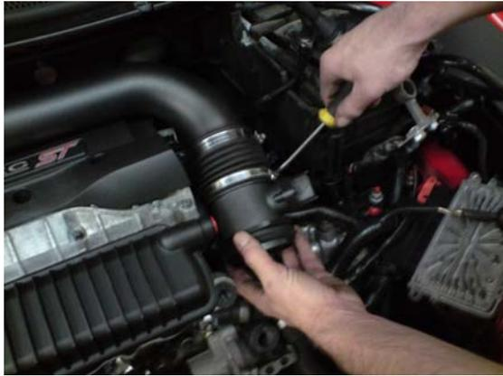
**14.** Remove the standard boost pipe by removing the 10mm bolt on the back of the pipe and the jubilee clip on the end of the pipe.
