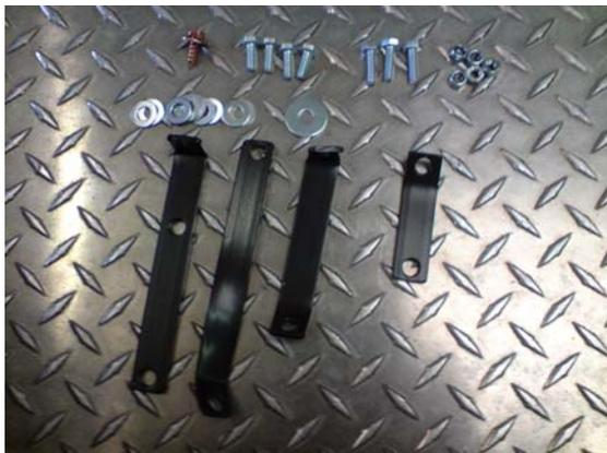
**16.** Fit the long bracket with a twist in it to the original hole in the cylinder head and then to the pipe, (leave loose until all of the kit is attached and ready for alignment)
