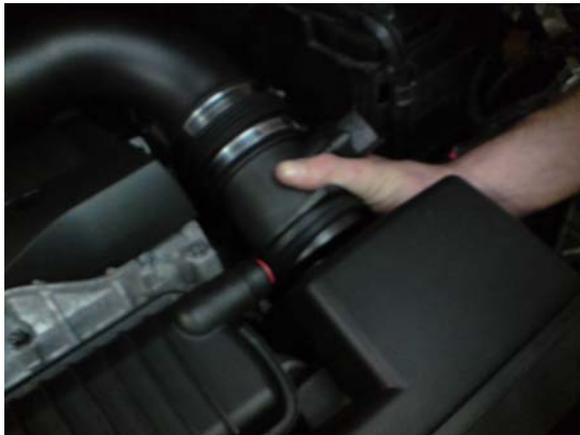
**12.** Slide the airbox out of the car to the right, be careful not to catch and damage anything when removing.
