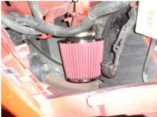
**27.** Once that the DSCI induction kit has been installed make final check to ensure that everything i.e. jubilee clips, brackets, pipes and connections have been tightened and nothing is chaffing.
