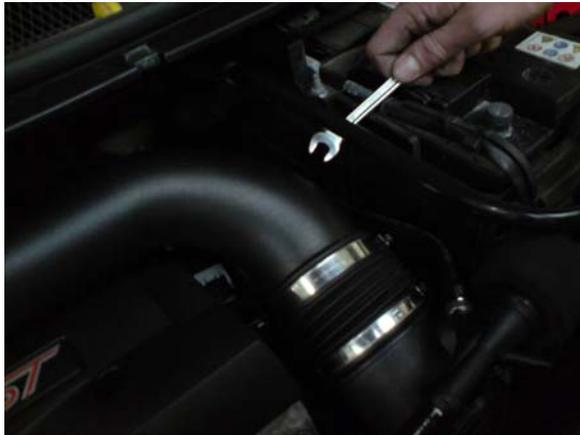
**11.** Pull MAF housing out of the standard airbox, remove seal from around MAF housing and keep in safe place as this will be needed if the standard airbox is to be re-fitted.
