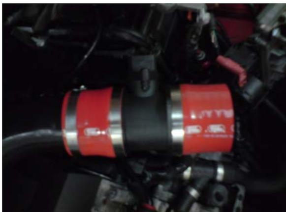
**22.** Remove nearside head light, this makes positioning and securing the second pipe and fitting the air filter easier. Before fitting the second pipe, you will need to remove the plastic guard from wiring loom and you **MUST** insulate using the insulation tape. There is also a small bracket on the gearbox that supports two earth straps, please make sure that this isn't touching the induction pipes, if so you may need to remove it.
