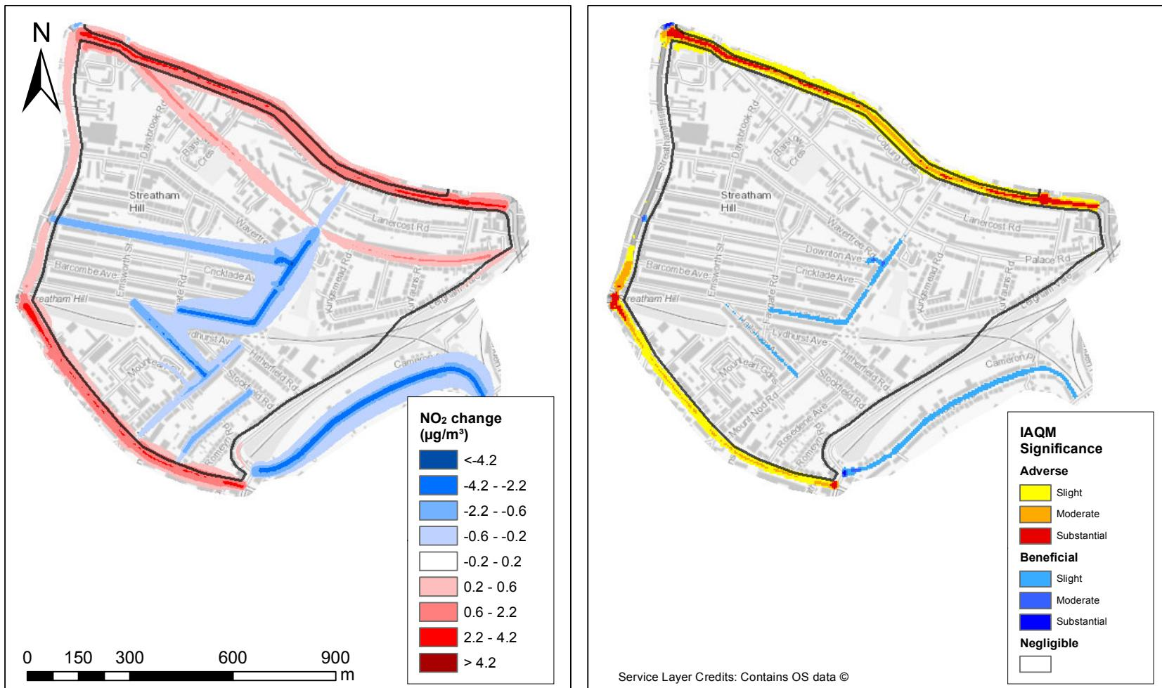
**Figure 6.12:** Difference plot (post-scheme minus pre-scheme) of annual average  $\text{NO}_2$  concentrations coloured by EPUK IAQM concentration change bands (left) and impact descriptor plot coloured by EPUK IAQM significance criteria (right), Streatham Hill LTN
