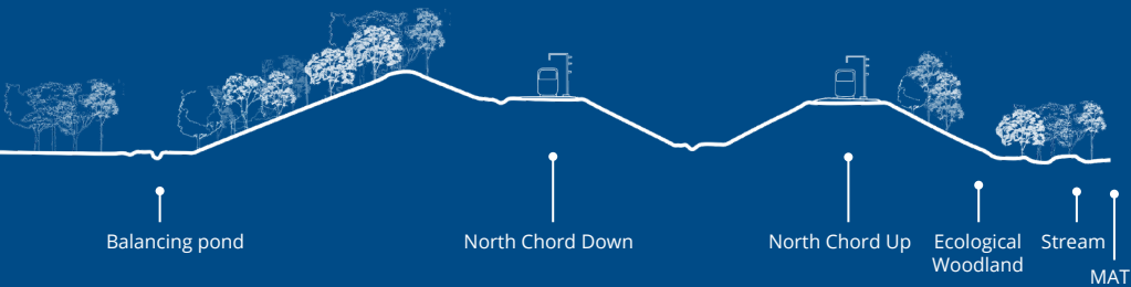
Section showing embankment and visual barrier above balancing pond MAT: Maintenance Access Track
