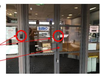
5. Deactivate the alarm, the panel is located immediately to the left of the entrance on the wall. Swipe the alarm fob over the panel as shown in the pictures. Once the alarm is deactivated, stay still until the sound stops and it is completely disarmed.
