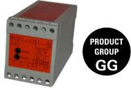
Foxtam AC current transducers can measure current either directly (max 7.5 Amps) or via the secondary of a current transformer, either 0-1 Amp or 0-5 Amp. The transducer converts the AC input current to an isolated analogue DC mA or DC voltage analogue signal output, directly proportional to the input. The 4KV isolated output signals can be utilised for many applications and can be fed into analogue meters, digital meters, PLC's or BMS systems.
