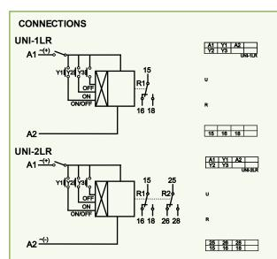
NOTE: A 4PCO 8 Amp latching relay is also possible utilising function I on our multi function unit UNI-4M. This unit is only with the ON/Off toggle input. And if you require a plug in unit see page 8.
